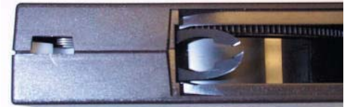
The tape cartridge leader has broken, or
