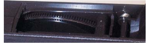
The tape cartridge leader has been rewound into the cartridge,
